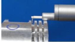
The surface measurement is not limited to roughness parameters. In the measurement of the scratches, the pickup is expected to rotate 90 degrees and skips along the arc. TIME®3231, with high resolutions and good straightness, achieves the breakthrough to access the profile information of small scratches.
