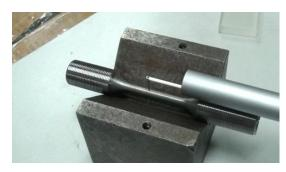
**Tensile Test Bar Measurement**
