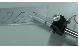
Scratch Depth & Width Measurement
