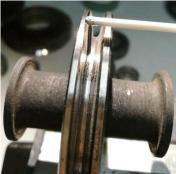
Narrow Ring Measurement Narrow Groove Measurement
